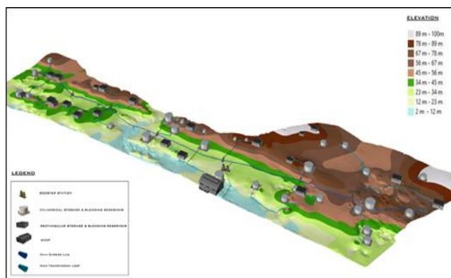
Figure 4: 3D view of Main Carrier, Transmission mains, Blending Reservoirs and Pumping/booster stations.
